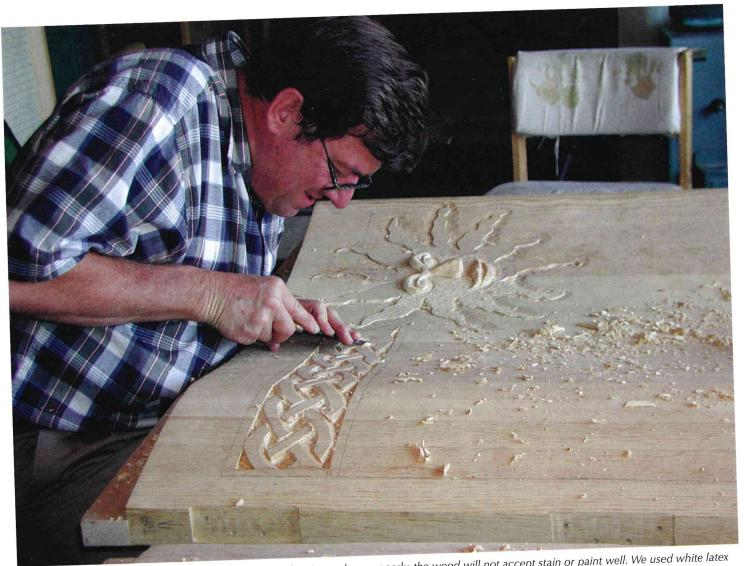
The carving and sanding were done by hand. If the sanding is not done properly, the wood will not accept stain or paint well. We used white latex underbody paint wiped on and off to create a whitewashed effect, followed by a coat of clear satin acrylic varnish.
