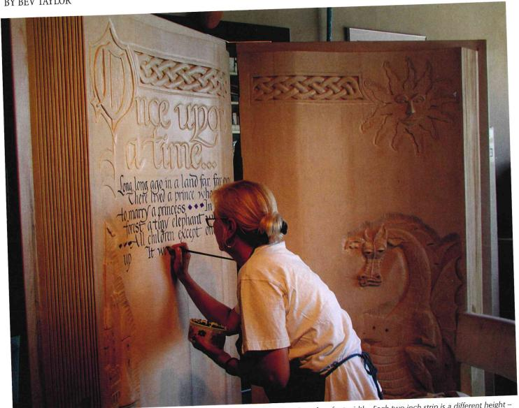
The doors are made of two-inch strips of clear pine laminated together vertically to form four-foot width. Each two-inch strip is a different height – ranging from two inches to five and a half inches - to replicate the curve of open book pages.
